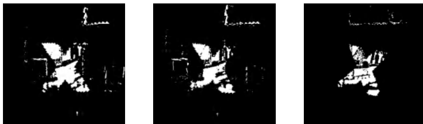
Fig. 12. Moving and grey level changing pixels between the log-polar images in the sequence and the panoramic background image. From left to right, the moving pixels corresponding to frames 1, 5 and 15 in the sequence
