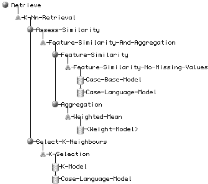
Fig. 7. A Configuration of a CBR application, where balls represent tasks, triangles represents PSMs and containers represents domain models.
