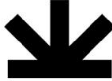
Fig. 2. Test chart for the derivation of the point spread function.
