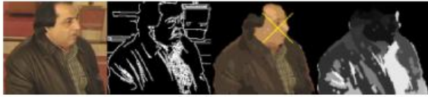
Fig. 2. Original image, contour image, quantization, initial regions.
